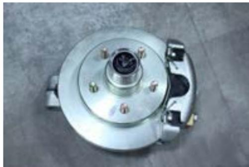
To check your bearings, raise your wheel clear of the road surface (by the procedure indicated in "tire changing"). With your hands on the outside edges of the tire, try to rock the wheel by pushing on one side and pulling on the other. No noticeable rocking should occur. Spin the wheel and listen for noise or roughness. A smooth, silent operation means that your bearings are in good order. If a grinding sound is heard, contact your SKEETER Dealer for warranty and or replacement instructions.
