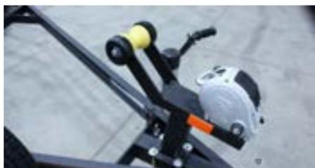
Maintenance of the mechanical winch is simple. Keep clean, lubricate regularly and apply heavy grease to the gears frequently. Make sure the winch line, strap or cable doesn't rub against anything sharp; fraying and wear could result. If your line, strap or cable becomes worn, contact your SKEETER Dealer for replacement as soon as possible.
